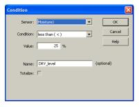
When setting the control conditions, it is useful to give a name to the threshold level ("DRY\_level" in this example). You will then be able to adjust the thresholds later without starting and stopping the program (this feature requires DeltaLINK version 2.4 or later).
