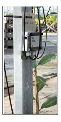
Pass the cable from the SM300 through the cable gland and connect to Channel 1 as shown (order for channel 1 is red, grey, white, black, green and blue):
