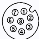
BF5 analogue output connector pin-out (looking into the cable at M12 connector end)
