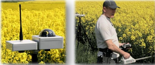
Illustration showing use of a BF5 mounted above a crop on a tripod along with a SunScan Radio Link
