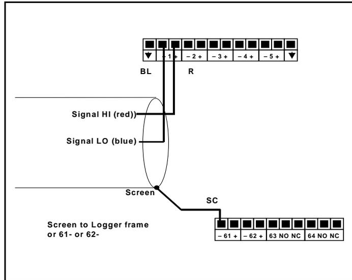
The example shows the ES2 sensor connected to analogue channel number 1 (for convenience) in the DL2e logger, with the following assumptions:
