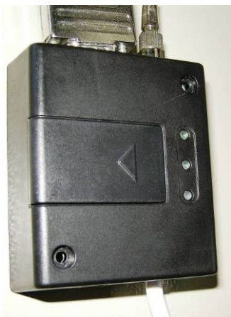
Figure 1 A GSM modem with DB9 RS232 connector top left, antenna connector top right and a power cable at bottom
