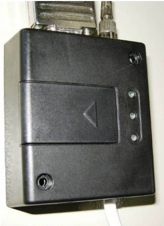
Figure 6 The GSM modem with DB9 RS232 connector top left, antenna connector top right and a power cable at bottom
