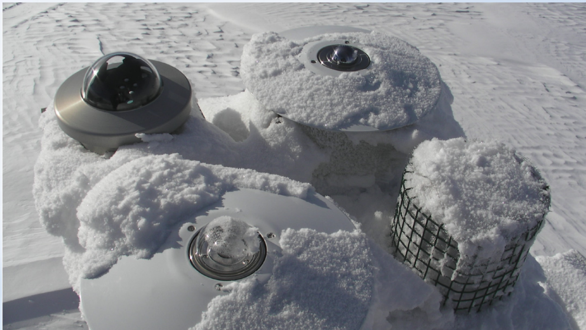
Figure 3. SPN1 radiometer (upper left), ventilated Eppley PSP radiometer lower left and a ventilated Eppley pyrgometer (upper right). A thin layer of frost is clearly visible on the PSP's dome.
