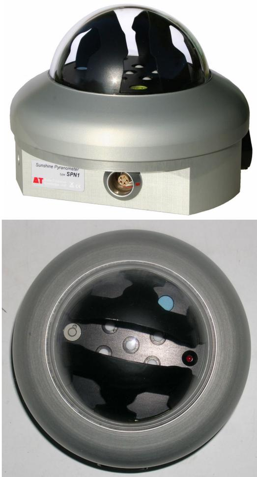
Figure 2: Side and top views of the SPN1 radiometer.
