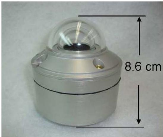
Figure 1: Side view of the modified Kipp and Zonen CM-22 radiometer used for RACORO.
