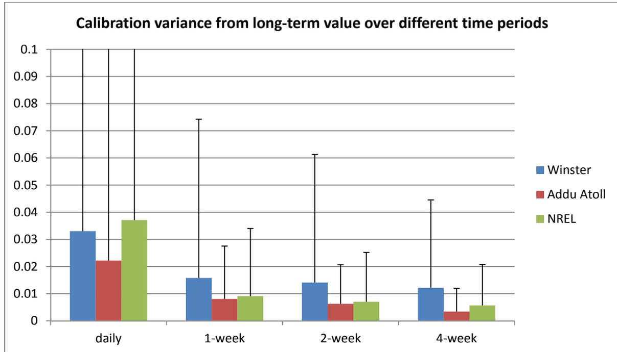
Fig.9 Calibration variability over time period and season (Box gives standard deviation, whiskers the worst case over the dataset)
