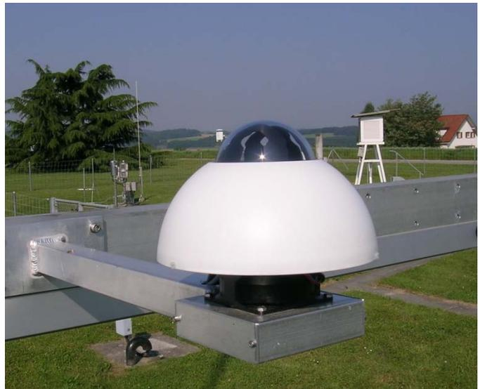
Fig.3 – SPN1 in MeteoSwiss ventilator
