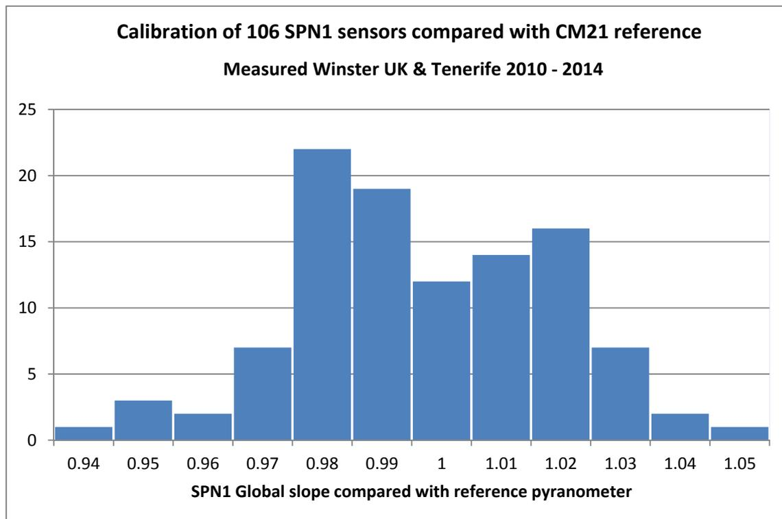
Fig.4 – SPN1 Calibration distribution – data supplied by manufacturer
