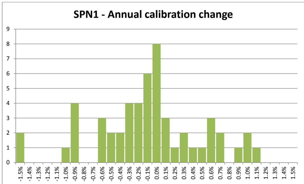
Fig.5 – calibration drift in % per year – data supplied by manufacturer
