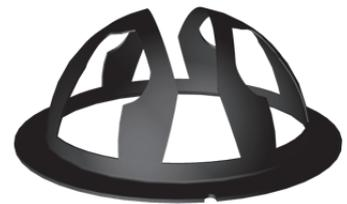
*Computer-generated shadow mask within the SPN1 ensures that one of the 7 thermopiles is always exposed to the full solar beam and one is in full shade regardless of the sun's position.*
