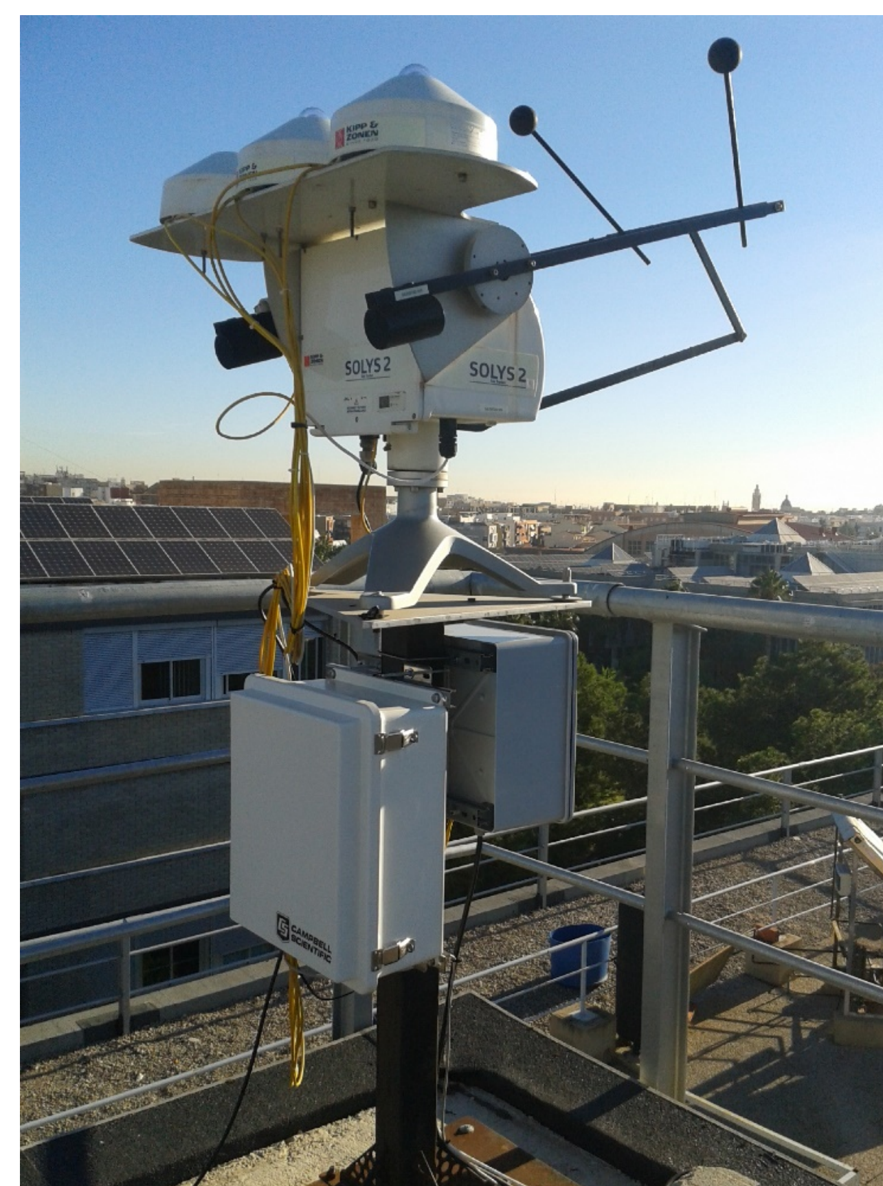
Figure 3. CMP21 and CHP1 radiometers on Solys tracker
