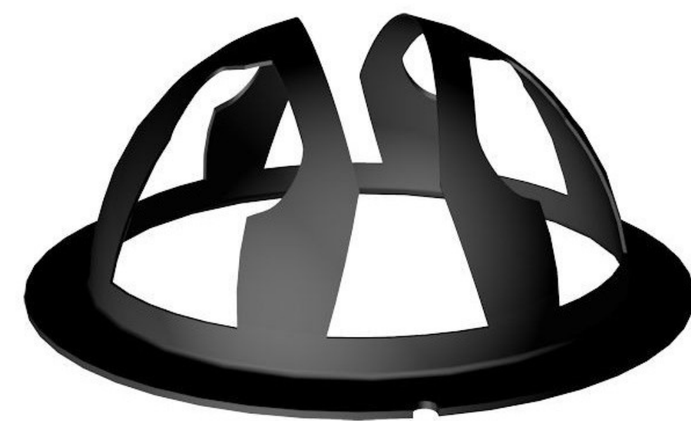
Figure 1. Radiometer SPN1 (up, scale ~1:1) with a detailed view of the computer generated shadow mask (right) and the 7 thermopiles distributed on a hexagon.
