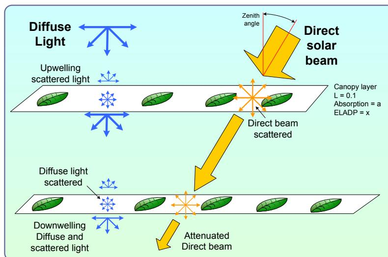
Figure 1 The canopy light scattering model used in SunScan
