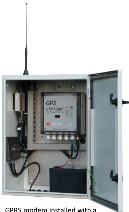
GPRS modem installed with a GP2 logger controller in an M-ENCL-B2 metal enclosure with SOL-4 solar power charger/regulator and LBAT4 battery.
