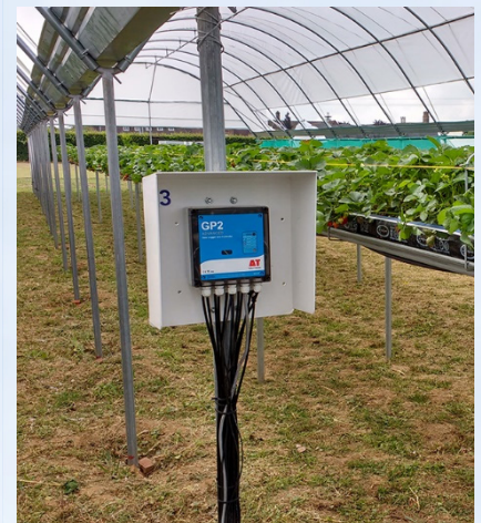
GP2 Data Logger installed at the NIAB EMR WET Centre research facility
