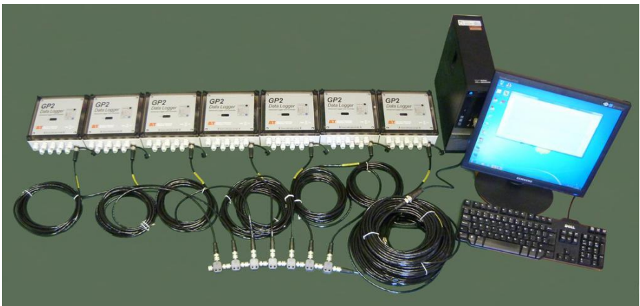
Figure A4 A network of 7 GP2 loggers connected to a PC via a total 100m of EXT/5w-xx extension cables and seven M12 5-way T-Piece connectors. This is the maximum number of loggers and maximum cable length supported.
