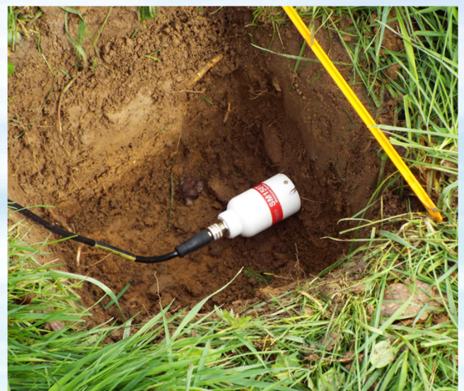
Figure 3. A Delta-T Devices SM150T Soil Moisture Sensor, installed at 20 cm depth at the Park Grass Experiment.
